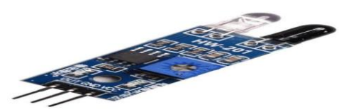
Fig IR Proximity Sensor
