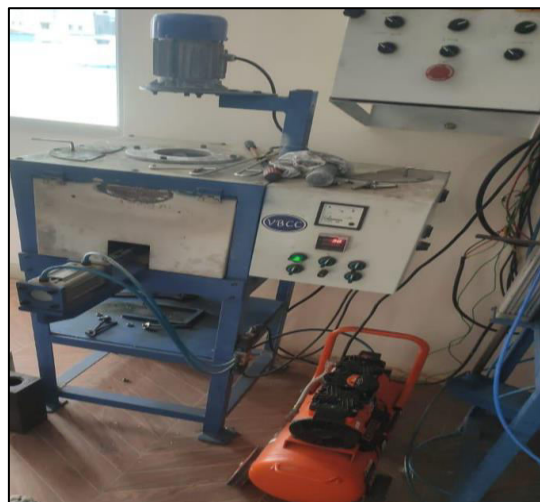
Figure 1: Stir casting setup for composite preparation.
