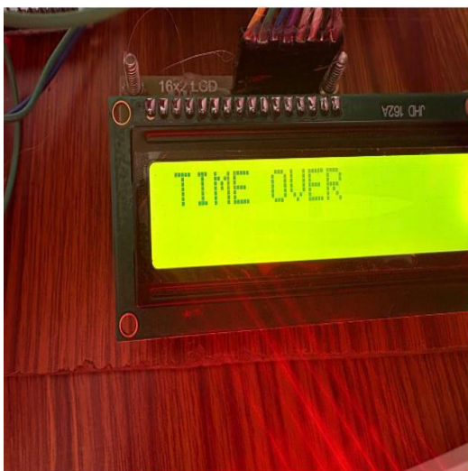
Fig: LCD Display Showing “Time Over” Status in RFID-Based Monitoring System
