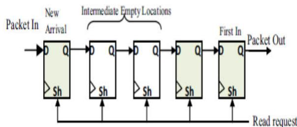
presents a conventional shift-register that is made offlip-flops. The data is written from one end and retrieved at other. The structure helps in synchronization of data between sender and receiver. However, the register can create bubble cells when the packet input and output rates are different. The design is simple but not suitable for NoC communications. To remove the problem of empty bubble, the arrival packet can be stored at the front empty cell rather than
