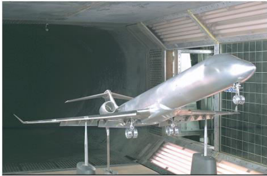
Figure 13: 7% scale full model of the CRJ-700 in IAR 6ft x 9ft atmospheric wind tunnel
