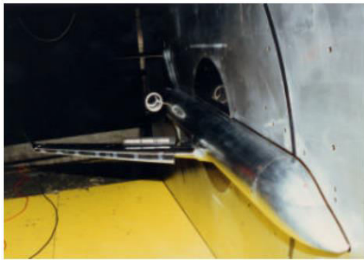
Figure 11: 7 percent scale half-model of the CRJ-700 installed in the IAR 5-ft high Reynolds number wind tunnel
