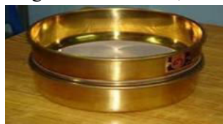
Fig- 3.3 Sieve used for find fineness of cement
