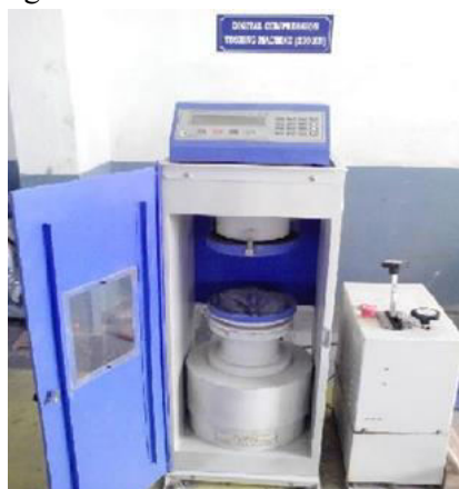
Fig. 4. 3 Setup for Compression Test
