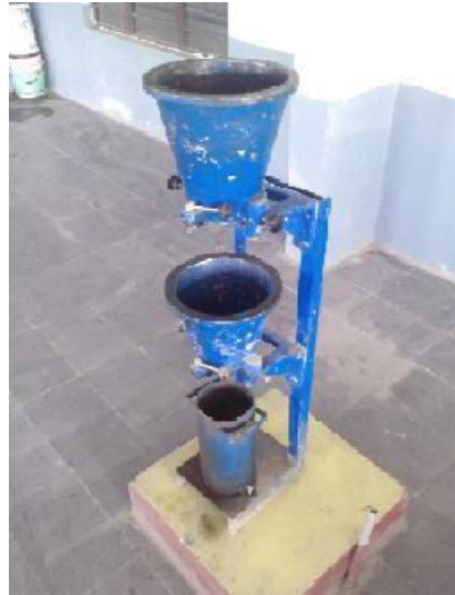
Fig. 4. 2 Apparatus for compaction factor test
