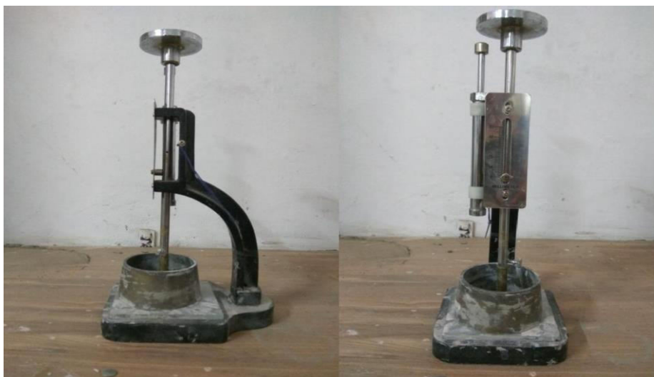
Fig 3.4-Vicat's Apparatus used for finding standard Consistency and initial and final Setting Times of Cement
