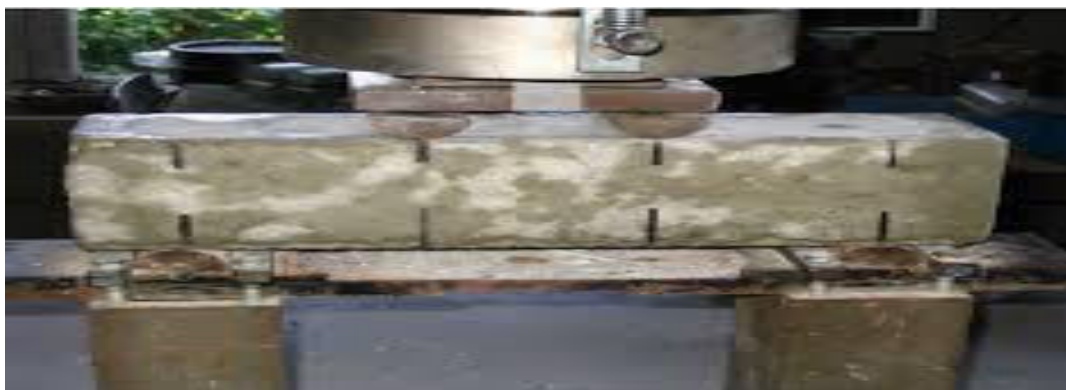
Fig 4.5 : Concrete Beam Specimen for Flexural Strength Test
