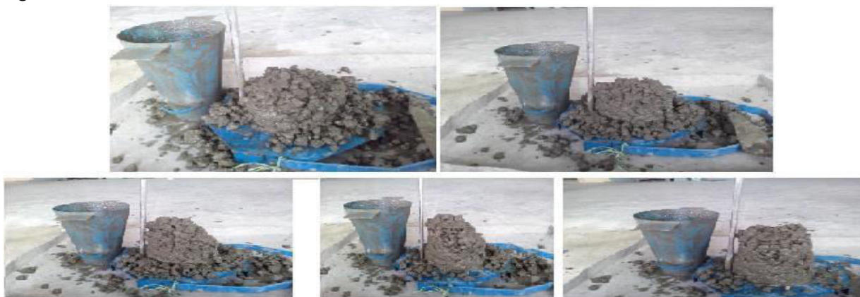
Figure 5. 1 : Slump results at MK+ MP 0%, MK+ MP 5%, MK+ MP 10%, , MK+MP 15%, MK+ MP 20%
