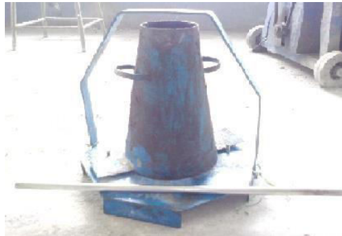
Fig. 4. 1. Apparatus to determine the workability of concrete ( slump test)
