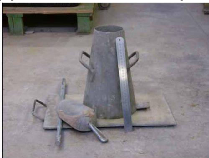
Figure 4.1: The Apparatus for Slump Test
