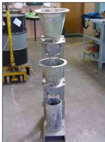
Figure 4.3: The Apparatus for Compacting Factor Test
