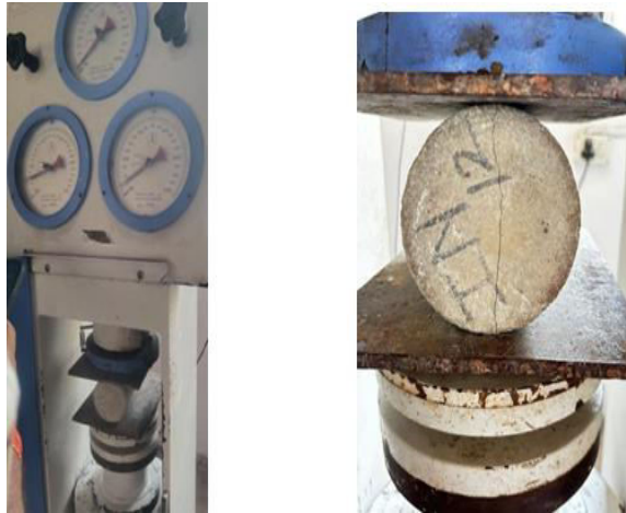
Split tensile test of cylinders
