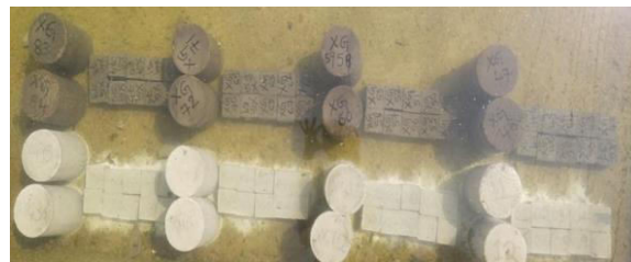
Curing of foam concrete samples
