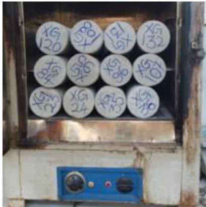
Placing the samples for oven drying
