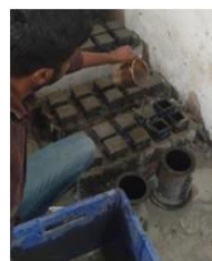
Casting of cube sand cylinders
