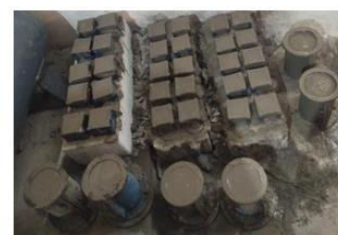
Casting of cube sand cylinders
