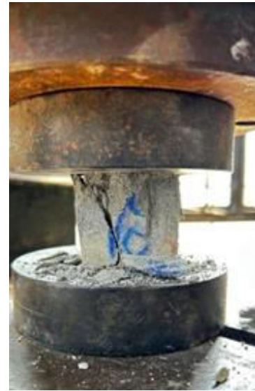
Cube under compression in UTM
