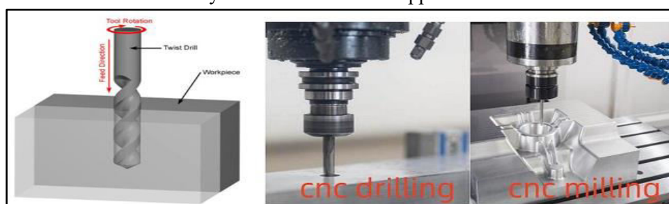
Fig 3: Working principle of CNC drill bit during drilling operation
